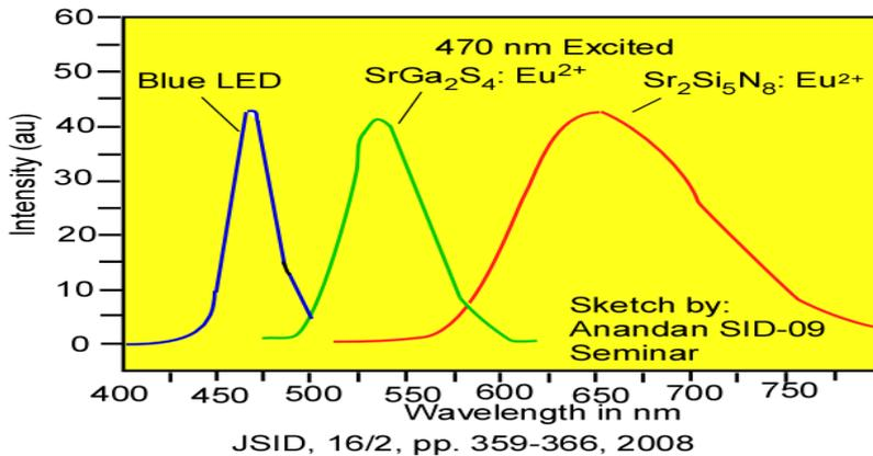
Fig. 5: Spectrum of Two-layer phosphor on blue-LED.
