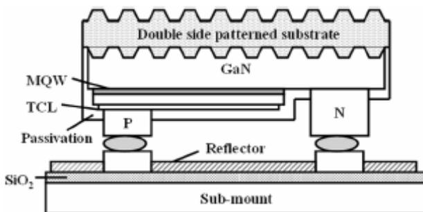
Fig. 7: Flip chip with double side patterned GaN for light extraction.
