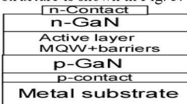
Fig. 3: Vertical LED structure with metal substrate
