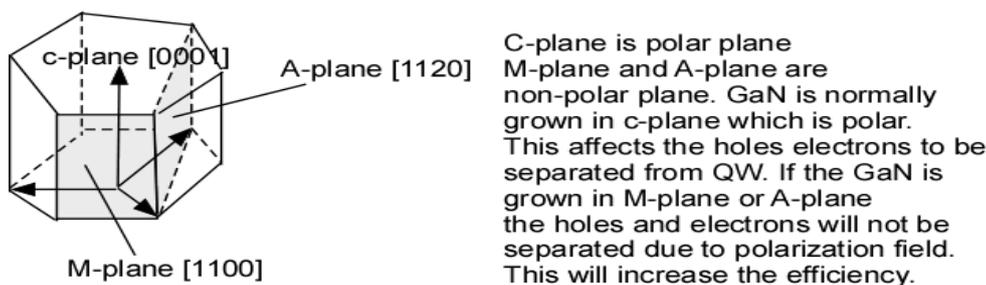
Fig. 1: Hexagonal crystal structure of GaN.
