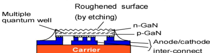
Fig. 4: LED-Flip-chip (Philips)
