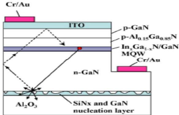
Fig. 6: GaN/Sapphire interface layer for light extraction.
