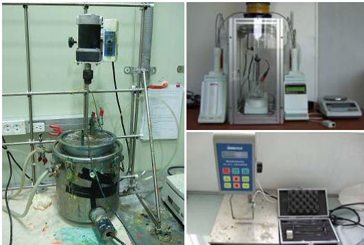
Fig. 3 Small-sized stirrer, NCO and viscosity measuring devices
