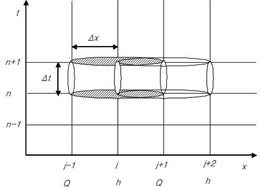
Figure 1. Schematic of the Abbott-Ionescu staggered scheme
