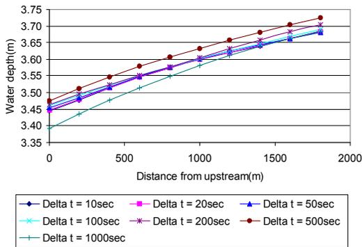
Figure 8. Water depth after 27000 sec with different time step
