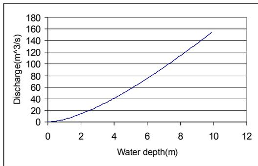
Figure 5. Downstream boundary condition (Rating curve)
