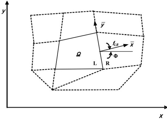
Figure 2. Geometry of Finite Volume  $\Omega$
