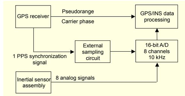
Fig. 1. Time synchronization scheme proposed in [5].
