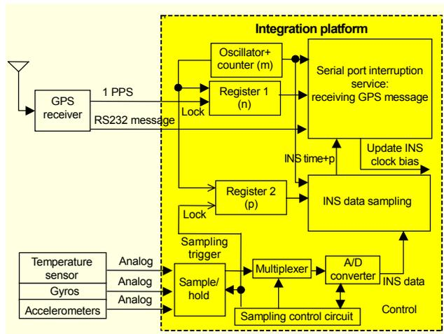
Fig. 5. Time synchronization with analog INS inputs.
