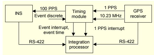
Fig. 2. Synchronization solution proposed in [8].
