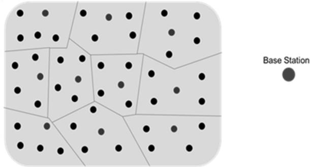
Fig. 3. The forming clusters with appointed cluster heads (the red dots are the cluster heads)
