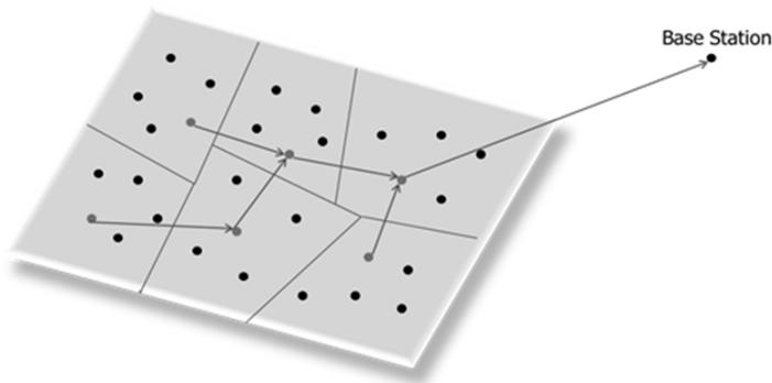
Fig. 1. Centralized base routing protocol Base Station Controlled Dynamic Clustering Protocol (BCDCP) routing path
