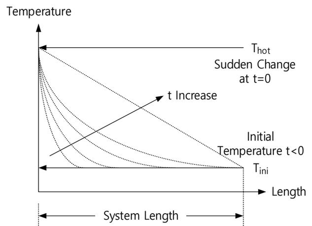
**Figure 2:** Predicted variation of a temperature profile with time. A sudden temperature increase is applied to the left surface of a system at  $t=0$ . Referring to **Figure 1 (b)**, the temperature gradient exponentially approaches a non-equilibrium steady state when the right surface is maintained at the initial temperature,  $T_{ini}$ .
