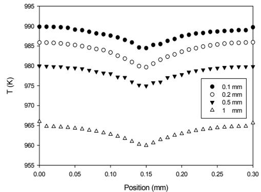
Fig. 6. Temperature profiles along the wafer surface,  $T_s = 873$  K and  $p = 10$  torr.
