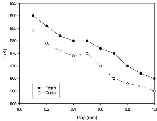
**Fig. 9.** Wafer temperature according to the gap size,  $T_s = 1003$  K and  $p = 10$  torr.
