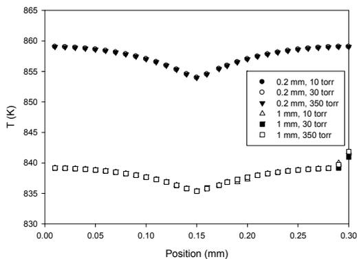
Fig. 5. Wafer temperature according to the gap size,  $T_s = 873$  K and  $p = 10$  torr.
