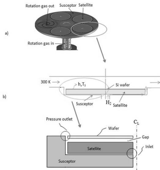
**Fig. 1.** Schematic representation of the domain under the study, (a) the whole susceptor and (b) detailed view with gap.
