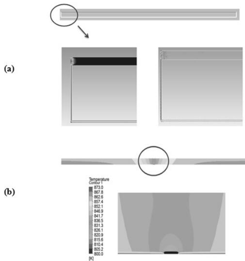
Fig. 4. (a) Velocity profiles and (b) temperature distribution when  $T_s = 873$  K and  $p = 10$  torr.
