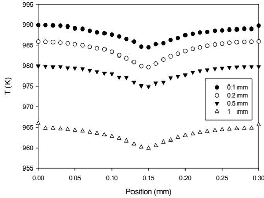
**Fig. 8.** Temperature profiles along the wafer surface,  $T_s = 1003$  K and  $p = 10$  torr.
