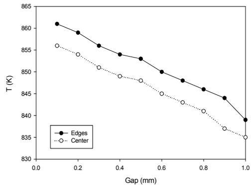
Fig. 7. Wafer temperature according to the gap size,  $T_s = 873$  K and  $p = 10$  torr.
