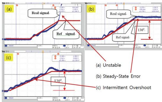
**Fig. 6.** Using the  $45^{\circ}$ (a),  $90^{\circ}$ (b) and  $120^{\circ}$ (c) controller respectively, at reference angle change from  $1^{\circ}$  ~  $130^{\circ}$ .
