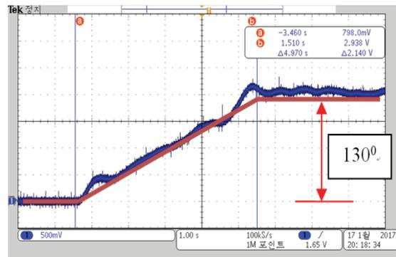
**Fig. 7.** Waveform output at a change controller with reference angle range in increment.
