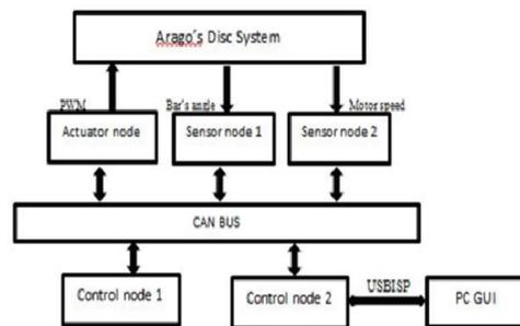
Fig. 2. Structure of a distributed control system with Arago Disc System.
