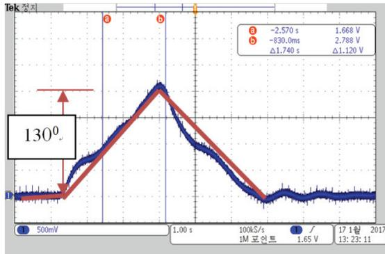
**Fig. 8.** Waveform output at a change controller with reference angle range in increment/decrement.
