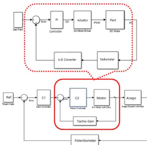
Fig. 3. A block diagram for explaining the inner (sub, speed) and main (position) controller.
