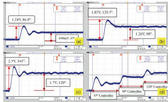
Fig. 5. Magnetic bar's angle of Arago's disc controlled at  $45^0$ (a),  $90^0$ (b),  $120^0$ (c), and change controllers with time(d).
