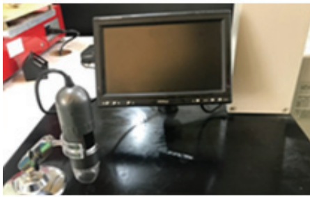
Fig. 3. USB microscope for measuring pore size.
