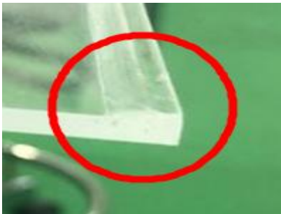
Fig. 10 manufactured wedge-type light guide plate
