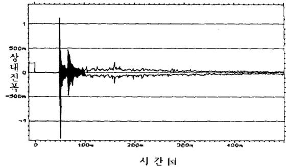
(b) Impulse response using electroacoustic system (Deutlichkeit: 0.71)
