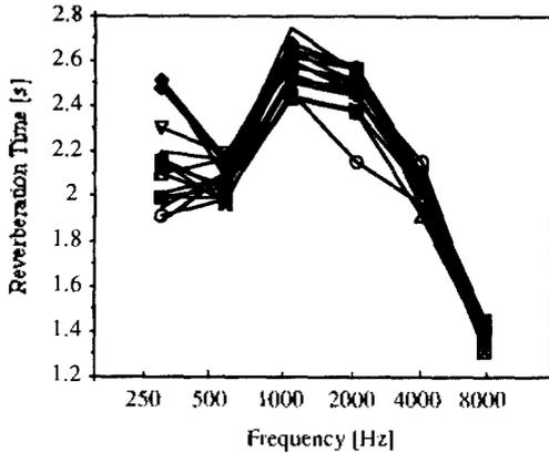
Fig. 1 The octave reverberation time at 24 receiver points.
