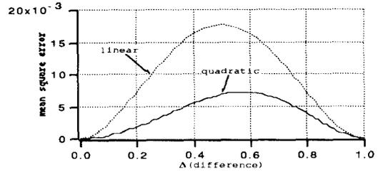
Fig3. Mean square error for interpolations of a white band-limited noise signal with  $f_c=0.125$  and  $B_b=0.25$
