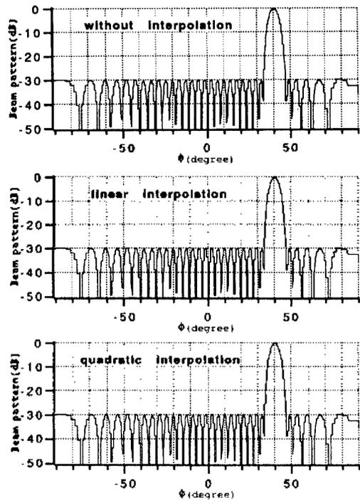
Fig.8. Beam patterns of interpolated beams in the case of narrow band signal for  $\delta_\theta = 1.0$ (steering angle  $\theta = 40^\circ$ )
