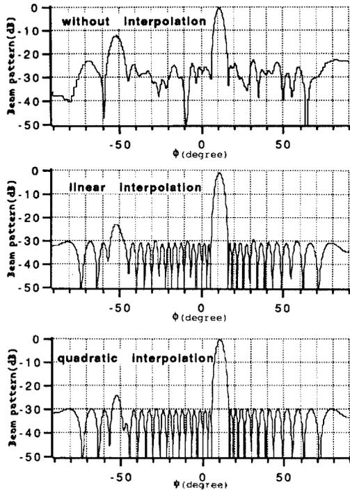
Fig.6. Beam patterns of interpolated beams in the case of narrow band signal for  $\delta_\theta = 0.3$ (steering angle  $\theta = 11.1^\circ$ )
