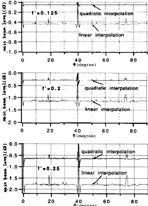
Fig.9. Main beam levels of interpolated signals in the case of narrow band signals with different center frequency  $f'$
