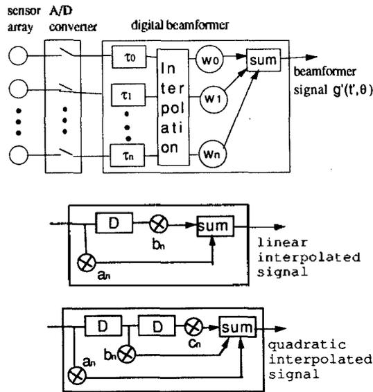
Fig5. Digital beamforming operation of interpolated signals
