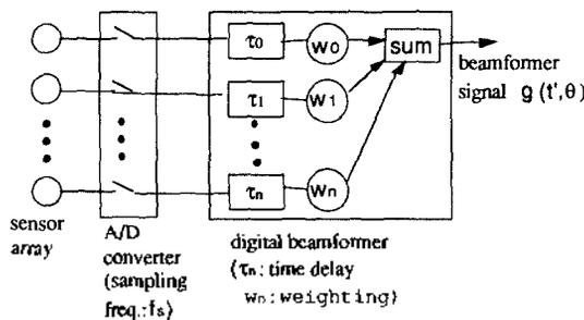
Fig1. Digital beamforming operation in time-domain
