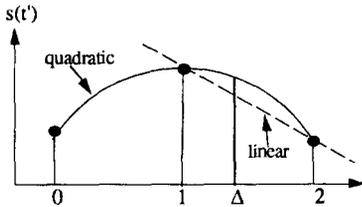
Fig2. Linear and quadratic interpolation
