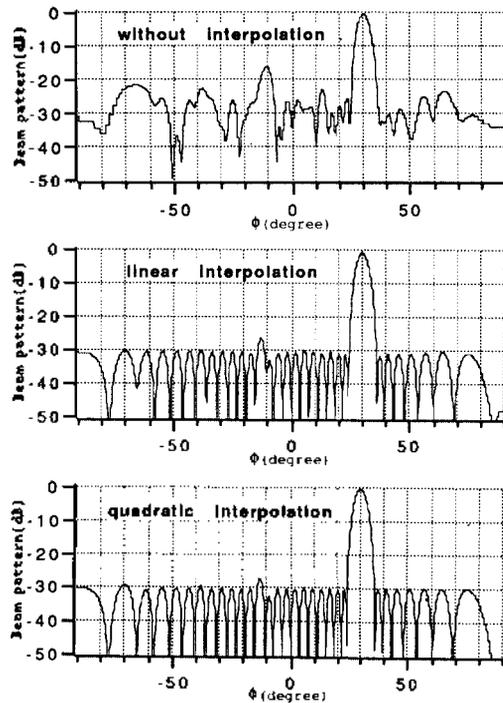
Fig.7. Beam patterns of interpolated beams in the case of narrow band signal for  $\delta_\theta = 0.78$ (steering angle  $\theta = 30^\circ$ )
