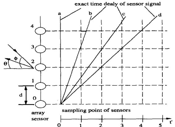
Fig4. Scheme of time-delay beamforming for linear array
