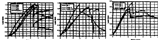
(a) Main Bush Bending (b) Main Bush Shear (c) Crossbrace Bending Fig. 6 Joint test results.
