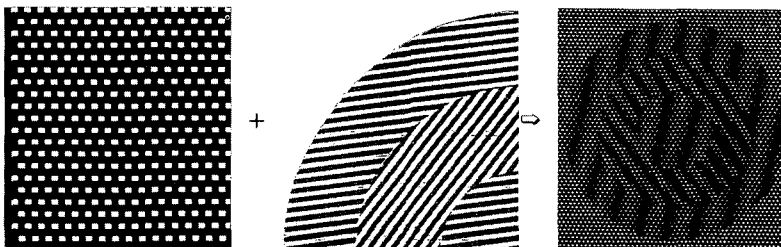
Fig. 3. Moire fringes resulted from overlapping transformed square grating with applied parallel line grating
