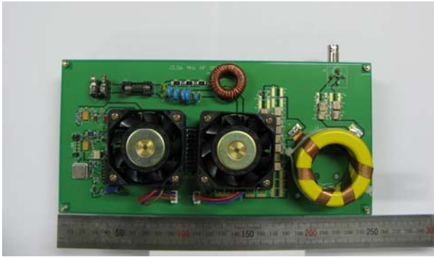
Fig. 4 Developed 13.56 MHz class E power amplifier circuit
