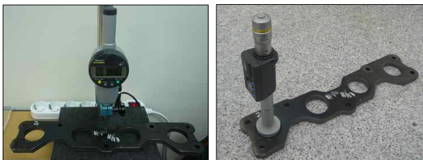
Fig.6 Flatness and hole size measurement of the plange
