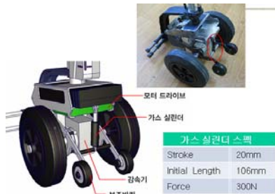
Fig. 7. Mechanism of the shock absorber
