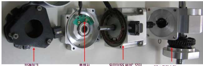
Fig. 5. SLOTLESS BLDC based actuator.
