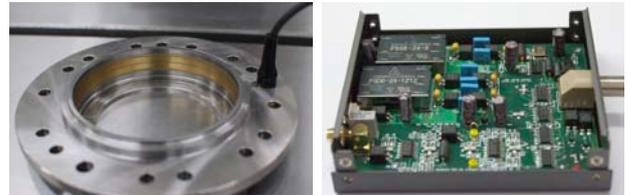
Fig. 2 1-axis capacitive displacement sensor and transducer
