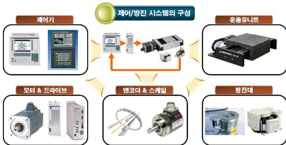
Fig. 1 Components of control/anti-vibration system
