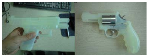
Fig. 5 Gun productions with SLA(Glock19 and 38caliber)
