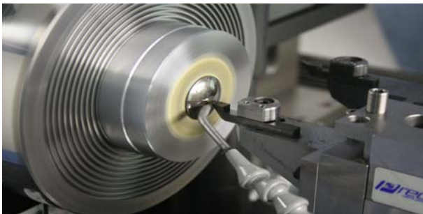
Fig. 4 Ultra precision machining of Ge lens
