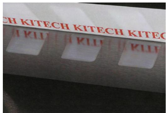
Fig. 2 Photograph of electro discharge machined surface
