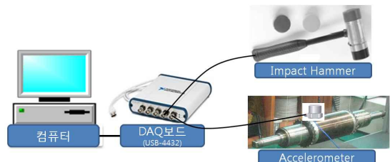
Fig. 2 Layout of Natural frequency inspection system
