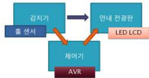
Fig. 2 Schematic diagram of Intelligent parking guidance management system
