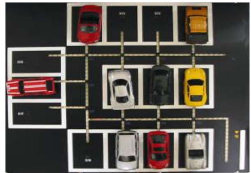
Fig. 1 Parking lot using LED guidance lamp
