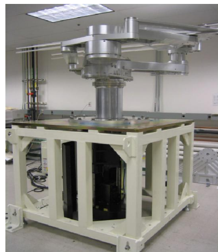
Fig. 1 Photograph of a LCD manufacturing machine with a bellows of a large diameter.
