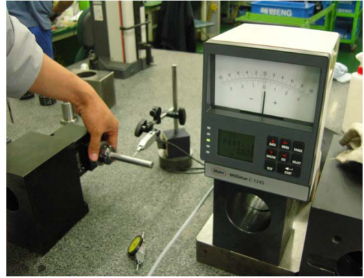
Fig. 5 Measurement of twisting deformation
