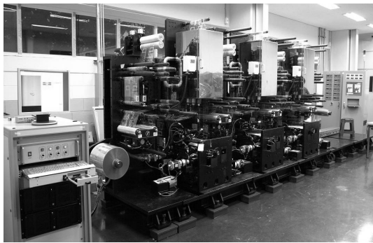
Fig. 3 Developed roll-to-roll printing system with multiple printing methods
