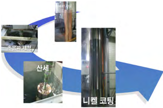
Fig. 3 Nickel Coating Process
