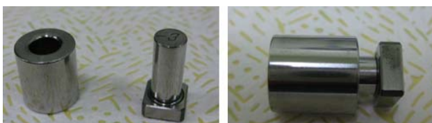
Fig. 6 Core and cavity alignment structure for secure of the tolerances in assembly
