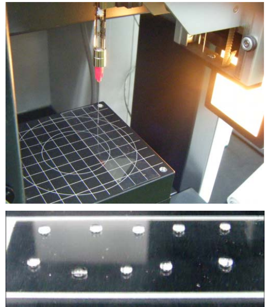
Fig. 3 Measurement of the contact angle for observing the surface energy
