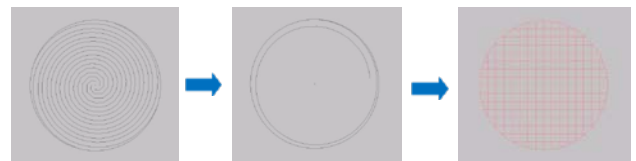
Fig. 3 Diagram of step of processing pattern using first idea in Copper 3-layer flexible PCB
