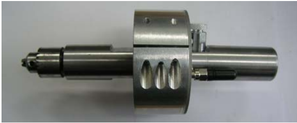
Fig. 4 Photograph of Drilling shaft
