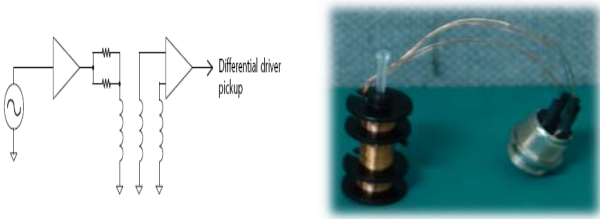
Fig. 3 Drive coil Type : Differential drive pickup
