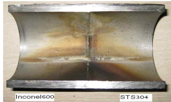
Fig. 1 Cross-section of welded pipe
