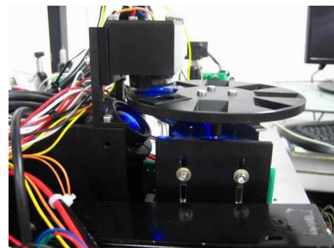
Fig. 2 Prototype of the fluorescence measuring sensor
