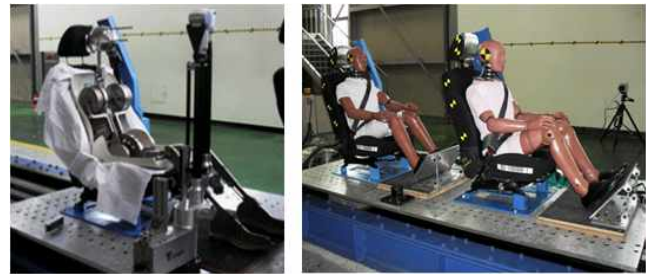
(a) Measurement with HRMD (b) Sled test Fig.6 Sled test
