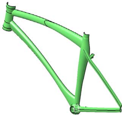
Fig. 2 Al6061 Bicycle Proto Sample
