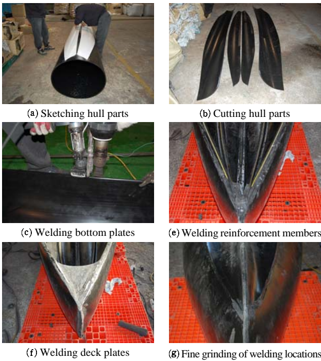
Fig. 3 Photographs of canoe building process by polyethylene plate welding method
