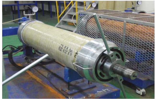
Fig. 2 Experimental set-up for long-term internal pressure test.
