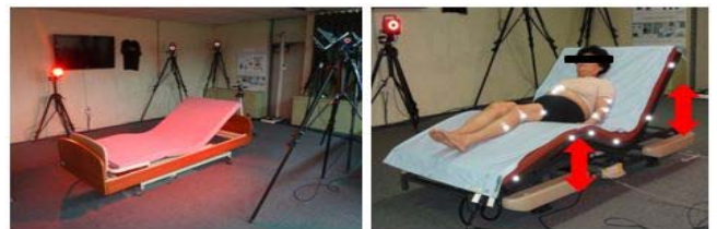
Fig. 2 Configuration of motion and pressure analysis experiments with VICON motion system and pressure measuring system
