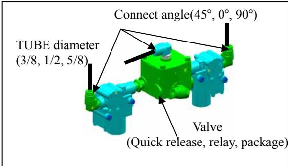
Fig. 3 Valve, connect (0°, 45°, 90°), tube diameter
