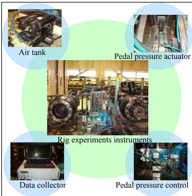
Fig. 1 Rig experiments instruments
