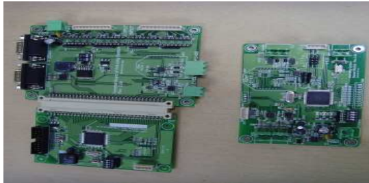
Fig. 3 PCB circuit for measurement & data transmission
