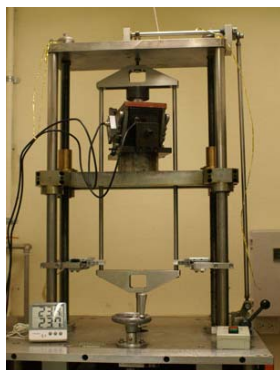
Fig. 4 Calibration for force sensor of starting block
