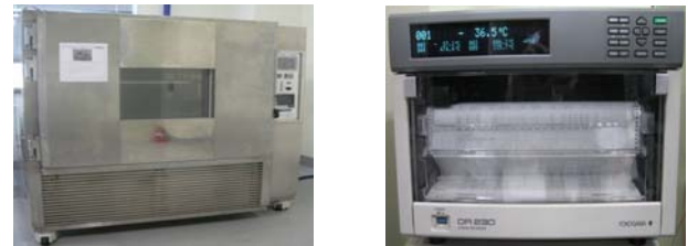
(a) Thermostat (b) Voltage-Temperature Recorder
