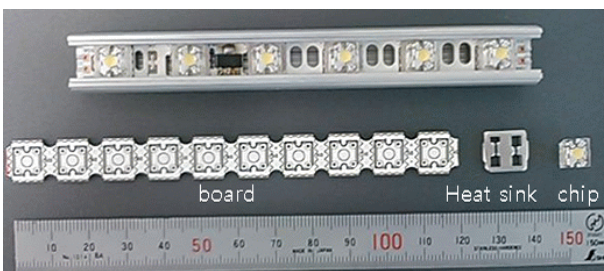
Fig. 1 Main components of the multi-chip LED package.
