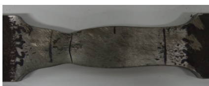
Fig.4 The specimen after tensile test
