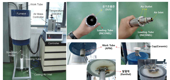
Fig. 2 Thermal fatigue test facility
