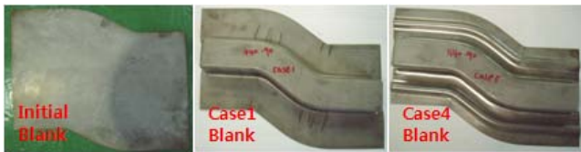
Fig. 5 Try-out process for rear case1 blank and case4 blank
