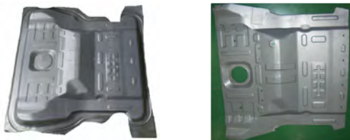
Fig. 6 Fabricated prototypes of rear floor panel
