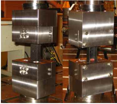
Fig. 4 Pictures of installed jig and specimen for test
